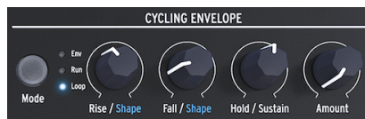
Der Cycling Envelope-Generator
