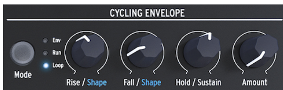
Der Cycling Envelope-Generator
