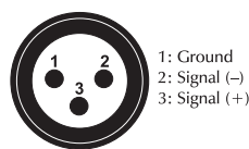
DMX-input XLR mounting-plug:
