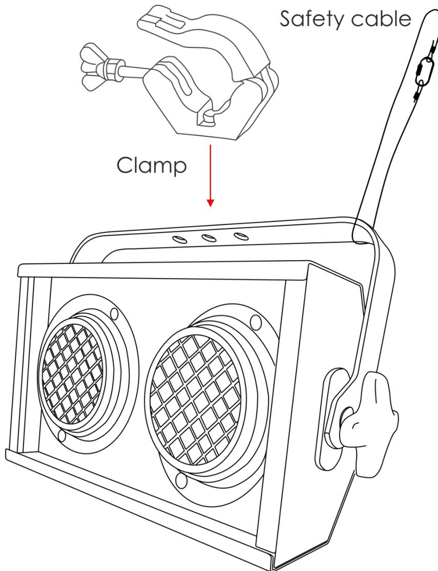
The Stage Blinder can be placed on a flat stage floor or mounted to any kind of truss with a clamp.
