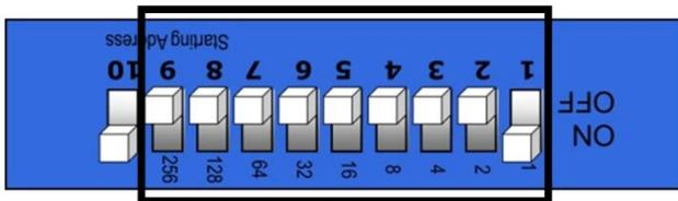
**Stand-alone:** Dip switch # 10 to ON position. Red LED on the backside of the Stage Blinder is ON.
