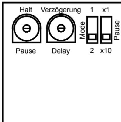
The duration of the station stop is set with the “Pause” switch and the “Pause” adjustment knob on the circuit board.
