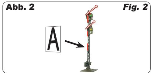
*Signals are marked with an alphanumeric combination. The name of the signal gives information about its position and direction of the route.*
