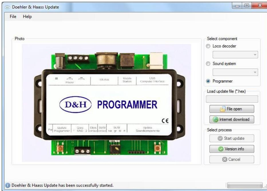
After the file has been loaded the programmer will be switched in the „Update operation mode“ pushing button T1 for e.g. 1.5 sec. The update process will be initiated by *Starting Update* and lasts about 3 seconds.
