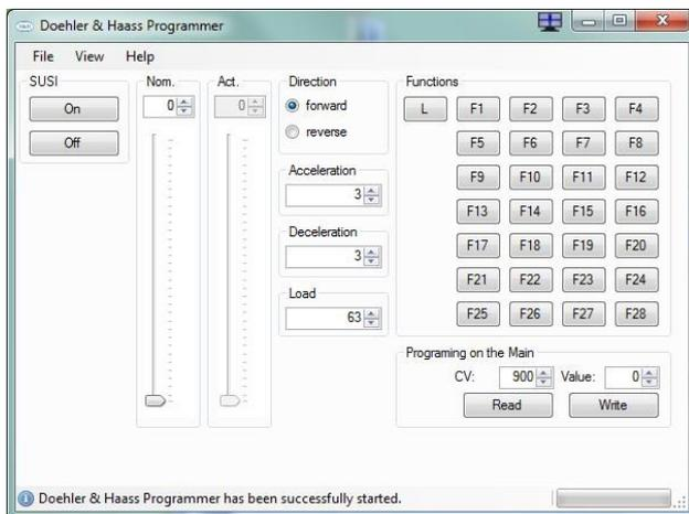
Actual speed level follows debit speed level by adjusted acceleration / deceleration and serves for the simulation of the decoder acceleration values (actual-speed level controller cannot be operated and serves only for displaying the currently issued speed level).
