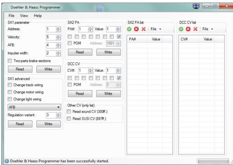
Decoder can be programmed in system formats SX1 / SX2 / DCC.
