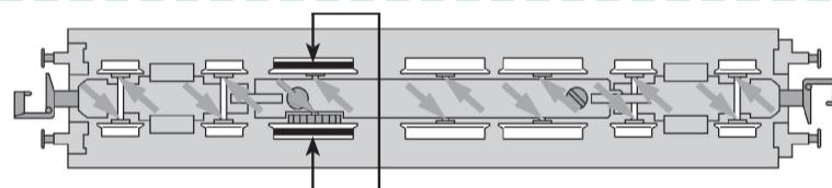
Lubrication: The motor and gear-box should only be oiled at the bearing points marked. Only use FLEISCHMANN oil 6599. Only put a tiny drop in each place (→), otherwise it will be overoiled. An applicator needle is located in the cap of the oil bottle for your use.
