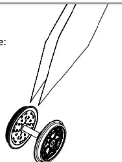
If used frequently, oil the wheelsets with a drop of non-resinous, acid-free sewing machine oil! In order to achieve the best possible running and traction properties, it is advisable to run the locomotive in for 25 minutes forwards and 25 minutes in reverse without load. Clean rails are essential for good performance.
