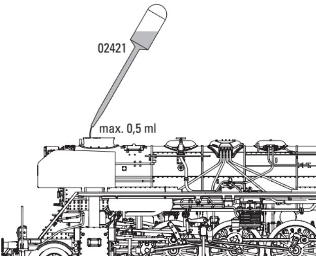
The smoke generator automatically shuts off after 5 minutes for safety reasons.
