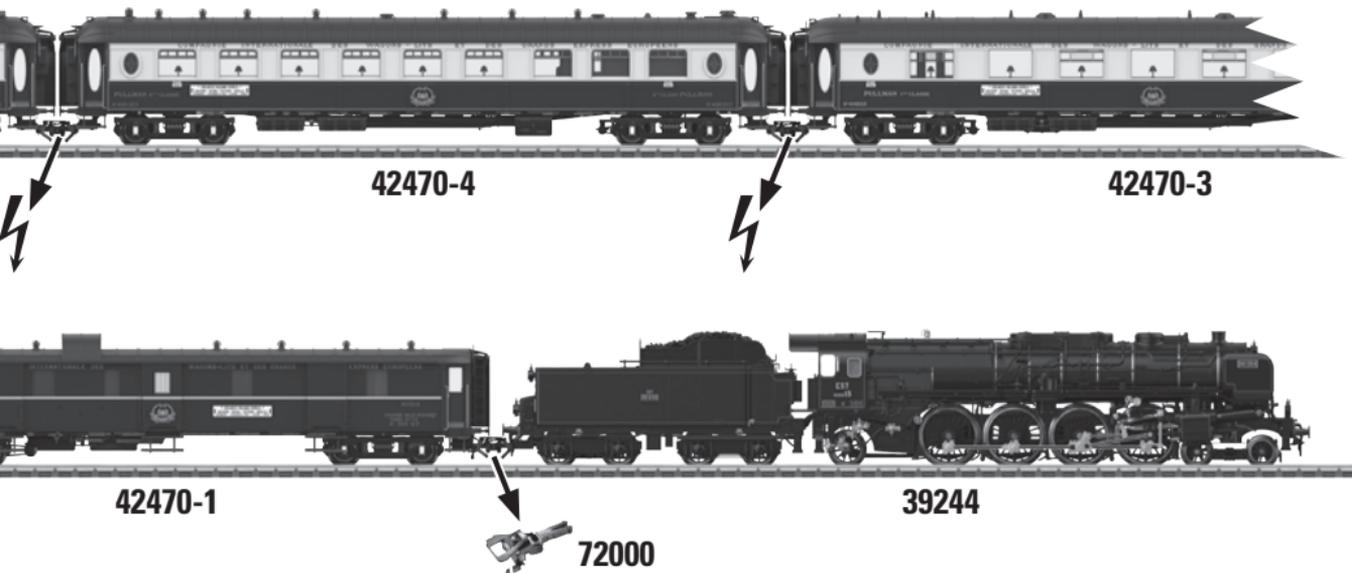
⚡ = stromführende Kupplung; current-conducting couplers; Accouplements conducteurs; Spanninggeleidende koppelingen; Conductoresde corriente; Conduitori di corrente; Strömledande kopplen; Stromforende koblinger
