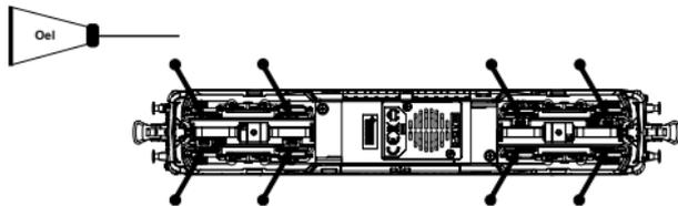
If used frequently, oil the wheelsets with a drop of non-resinous, acid-free sewing machine oil! In order to achieve the best possible running and traction properties, it is advisable to run the locomotive in for 25 minutes forwards and 25 minutes in reverse without load. Clean rails are essential for good performance.
