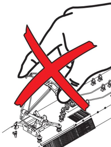
**Note:** Before running the locomotive for the first time, the pantographs must be unlocked by hand. The pantograph flexes upwards on its own in the upper position.
