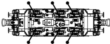
If used frequently, oil the wheelsets with a drop of non-resinous, acid-free sewing machine oil! In order to achieve the best possible running and traction properties, it is advisable to run the locomotive in for 25 minutes forwards and 25 minutes in reverse without load. Clean rails are essential for good performance.
